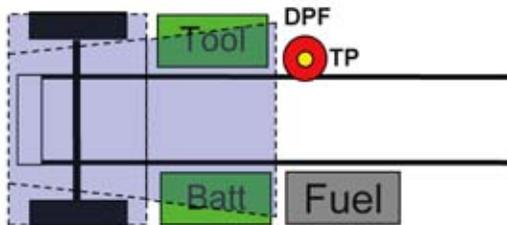
**D8** is used for vertical independent exhaust RH back of cab, including DPF, battery box LH under, tool box RH under and fuel tanks located BOC. Charts located on pages 3-41.
