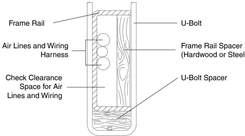
**FIGURE 4-8.** Clearance Space for Air Lines and Cables
