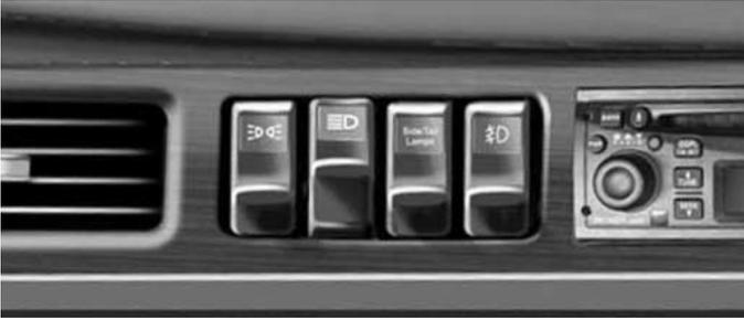
1. Remove trim bezel by prying upward at one of the four pry points. Carefully unzip the remaining clips
