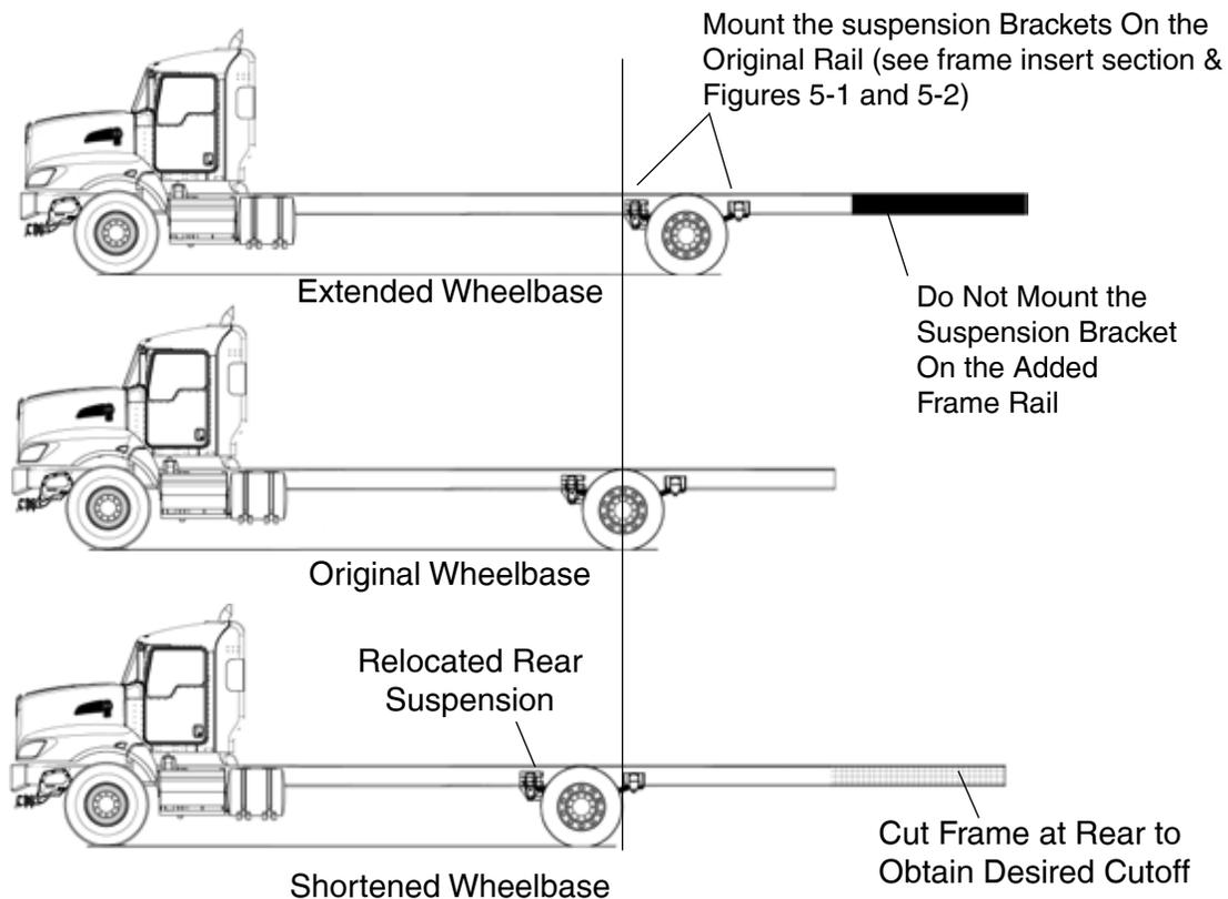
**FIGURE 5-3.** Comparison of Original, Shortened, and Extended Wheelbases.
