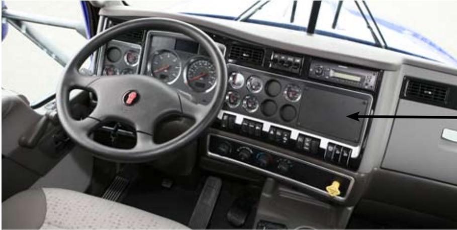
The T470 comes standard with a accessory dash panel - 7.5" x 5" (193mm x 128mm).
