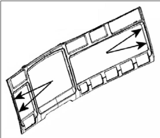
2. Remove (4) screws to remove Speedo - Tach panel.
