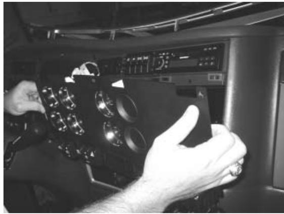
5. Unclip leads to gauges, effort is required to separate the friction lock.
