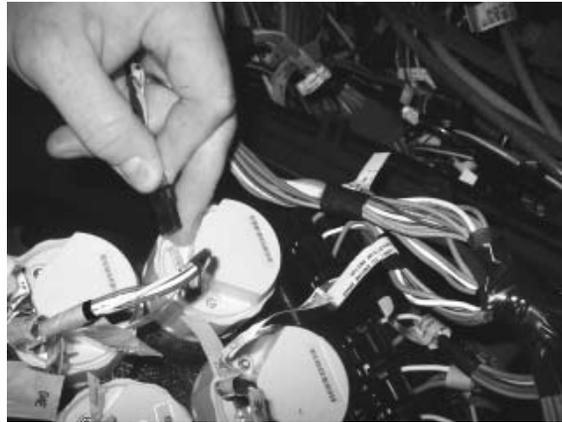
6. Pinch to unlock connector and remove right gauge panel.
