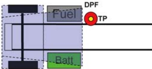
**D7** is used for vertical independent exhaust RH back of cab, including DPF, battery box LH under, and fuel tank RH under. Charts located on pages 3-40.
