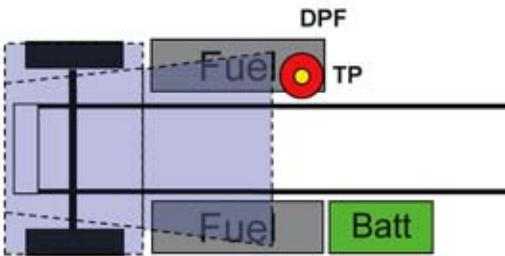
**D11** is used for vertical independent exhaust RH back of cab, including DPF, fuel tanks LH and RH under, and battery box LH BOC. Charts located on page 3-44.
