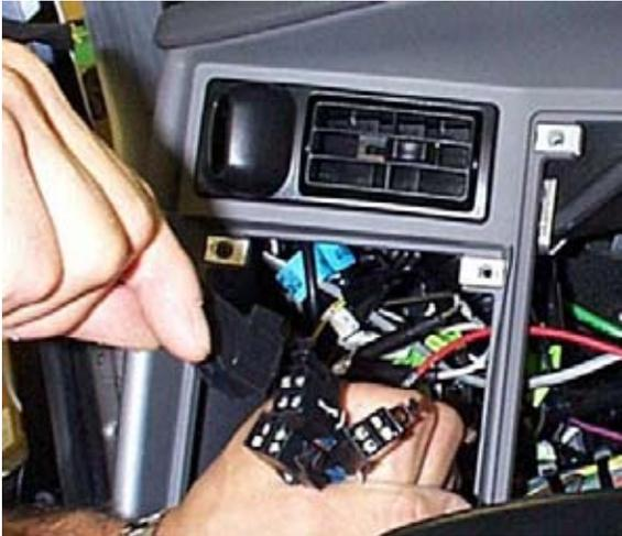
**FIGURE 6-13.** Spare Relay Connectors
