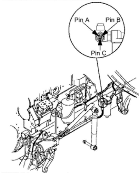
**FIGURE 6-7.** Fuel Filter Restriction Pressure Gauge Sensor Location (typical)
