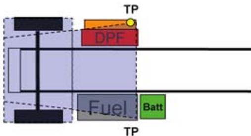
**D2** is used for single exhaust located side of cab with the vocational style battery box LH BOC, fuel tank LH under, and DPF RH under. Charts located on pages 3-35.
