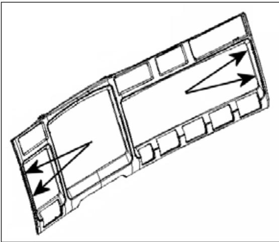
2. Remove (4) screws to remove Upper Switch Cluster.
