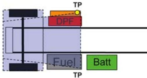
**D3** is used for single exhaust located side of cab with fuel tank LH under, DPF RH under and battery box BOC. Note: This layout can be used with a modular sleeper, dimensions will not change. Charts located on pages 3-36.
