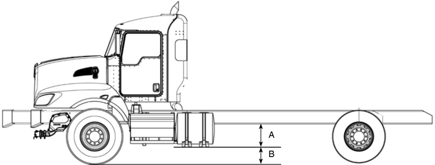
**TABLE 3-18.** Ground Clearance for Fuel Tanks
