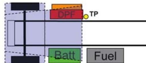
**D4** is used for single exhaust right hand (RH) back of cab with battery box LH under, DPF RH under and fuel tanks BOC. Charts located on pages 3-37.
