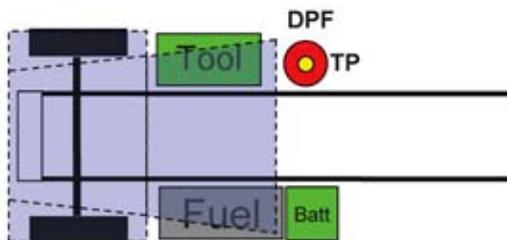
**D9** is used for vertical independent exhaust RH back of cab, including DPF, vocational style battery box LH BOC, fuel tank LH under and tool box RH under. Charts located on pages 3-42.
