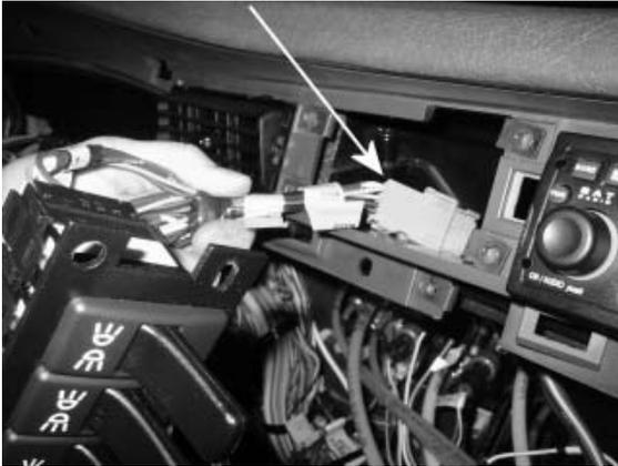
4. To remove switches push both tabs down...
