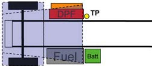
**D5** is used for single exhaust RH back of cab with vocational style battery box LH BOC, fuel tank LH under and DPF RH under. Charts located on pages 3-38.
