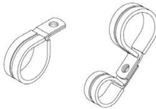
FIGURE 7-1. Clamp and Butterfly Clamp
