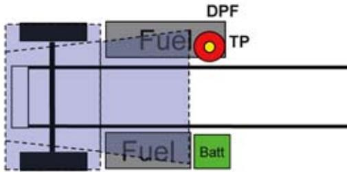
**D10** is used for vertical independent exhaust RH back of cab, including DPF, vocational style battery box LH BOC, fuel tank LH under and fuel tank RH under. Charts located on page 3-43.
