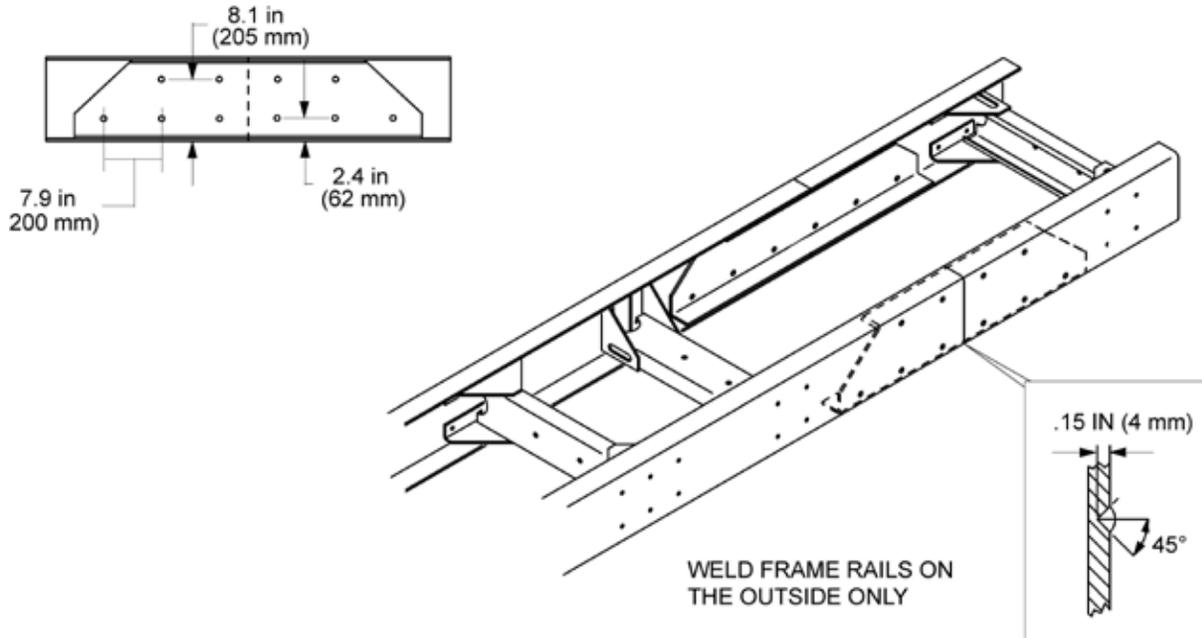
FIGURE 5-1. Detail of Frame Extension and Joint Welding
