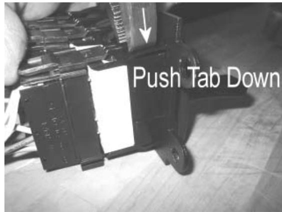
...and then push switch out of plate on top side...
