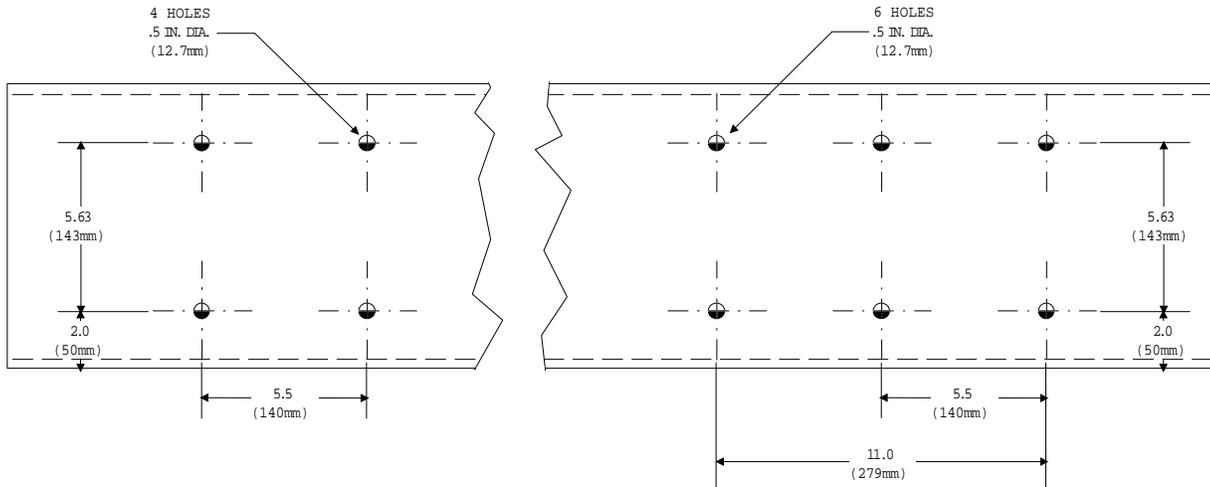
FIGURE 4-6. Crossmember-Gusset Hole Pattern Requirements. [inch (mm)]
