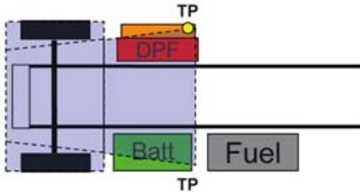
**D1** is used for single exhaust located side of cab (SOC) with battery box LH under, DPF RH under and fuel tanks back of cab (BOC). Charts located on pages 3-34.
