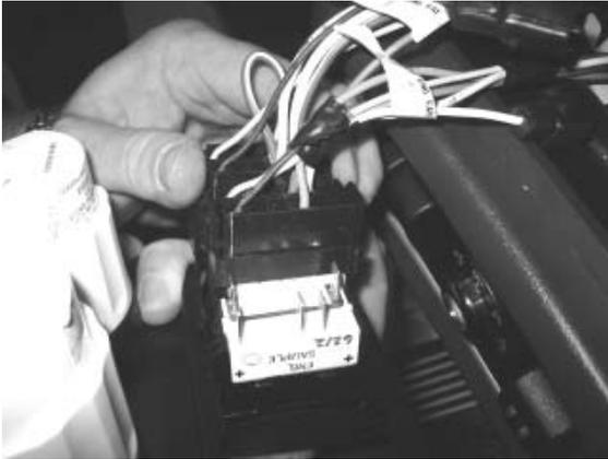
12. Unclip harness and remove left gauge panel.
