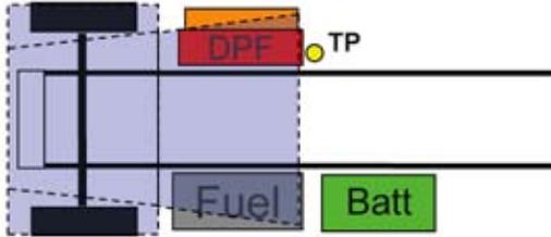
**D6** is used for single exhaust RH back of cab with fuel tank LH under, DPF RH under and battery box LH BOC. Charts located on pages 3-39.
