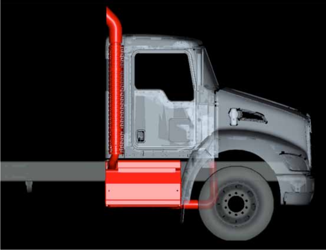
FIGURE 4-11: Right View of Right Hand Under DPF and SCR with Single SOC Tailpipe
