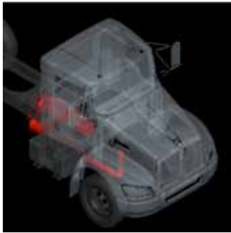
Horizontal DPF and SCR with Horizontal Tailpipe
