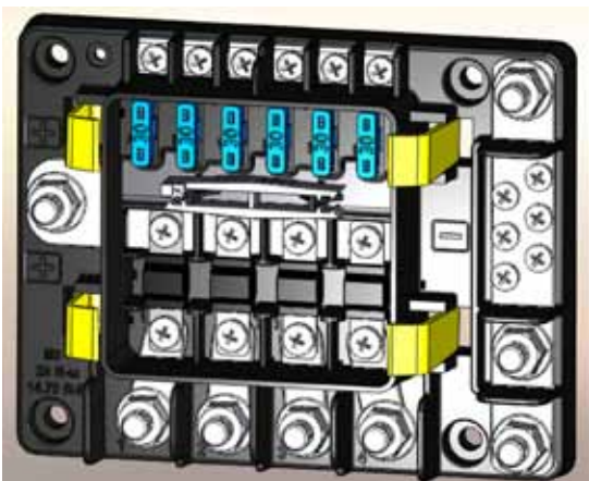
FIGURE 8-23. Detail of Body Builder Power Distribution Module
