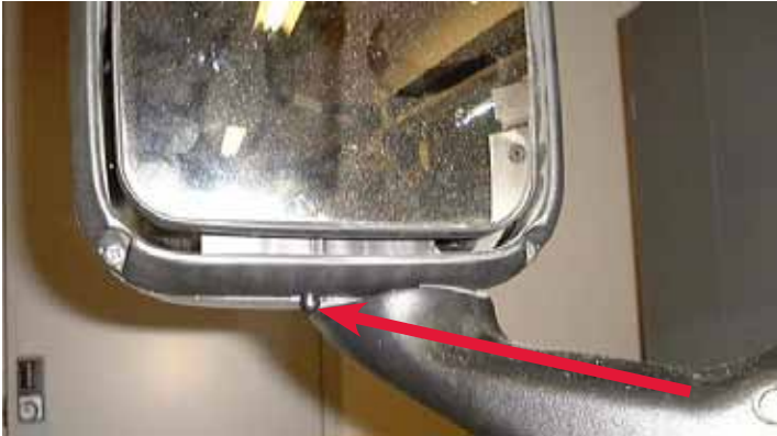
FIGURE 2-4: Aerodynamic Mirror OAT Sensor Location
