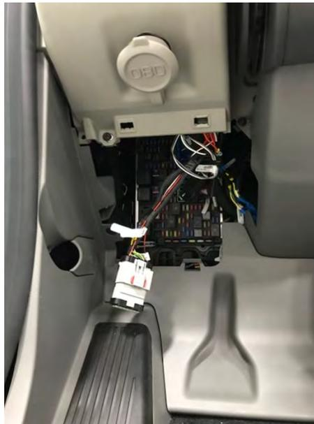
*Figure 99 RP1226 Connector Inside the Cab*
