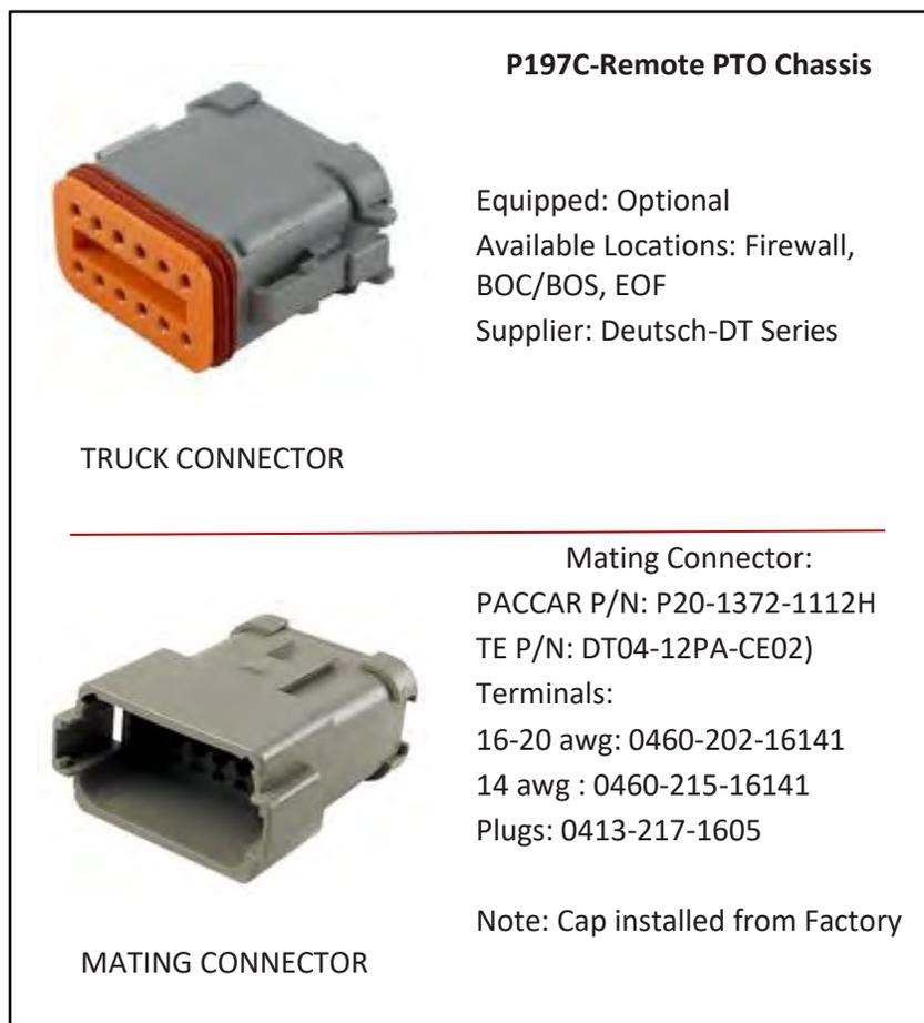
*Figure 59 12-Pin PTO Connectors (MX-only)*
