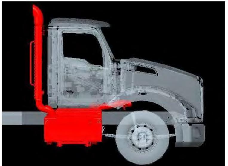
*Figure 108 Right Hand Under DPF/SCR on Daycab with Back of Cab Tailpipe*
