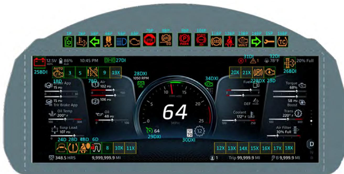
Figure 7 Digital Dash (15in) for T680/T880/W990 (EPA 2021+)
