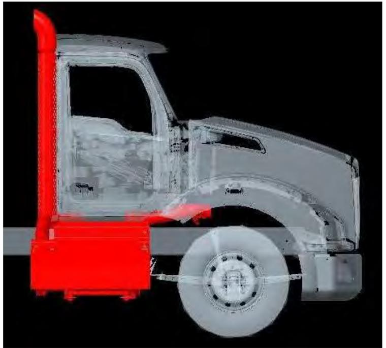
*Figure 107 Right Hand Under DPF/SCR on Daycab with Dual Side of Cab Tailpipes*
