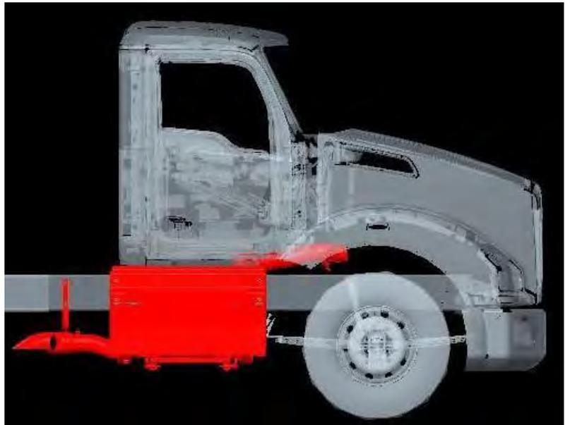
*Figure 109 Right Hand Under DPF/SCR on Daycab with Ground-Dump Tailpipe*
