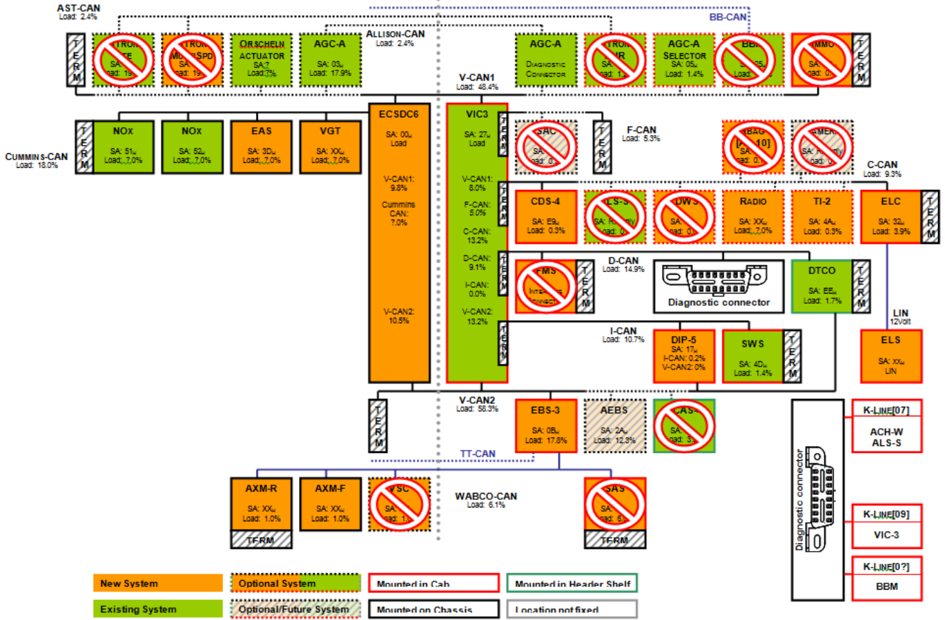
Figure 24 25 Data Bus Communication Architecture
