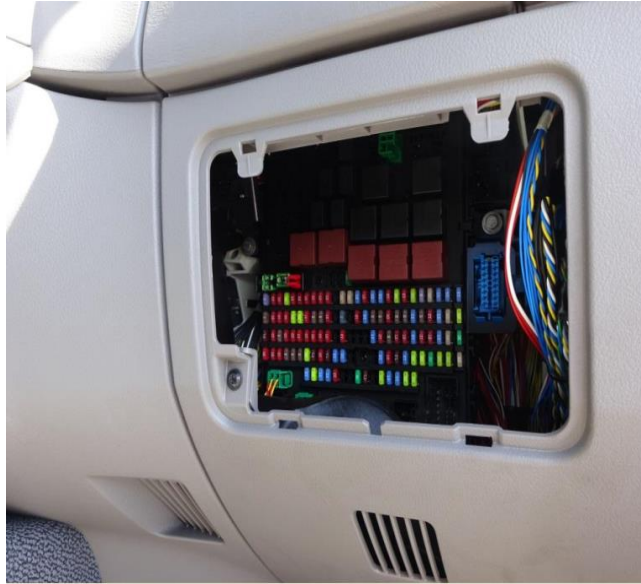
Figure 27 Inside View - Electrical Junction Box Location
