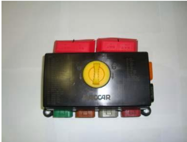
Figure 32 Power Distribution Center
