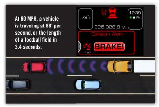
Far beyond a mere warning system, Kenworth collision mitigation detects when the truck may be about to collide with another vehicle or object, alerts the driver and takes pre-emptive braking action—when necessary—to avoid or considerably reduce the severity of a crash.
