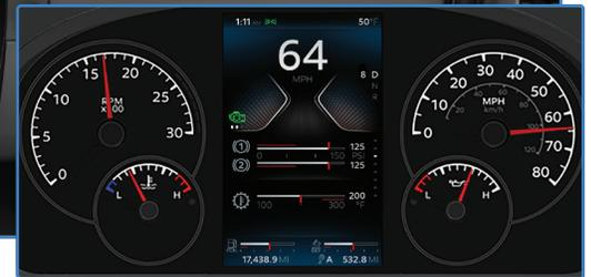
Standard Instrument Panel with 7-Inch Digital Display
